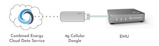
A compatible USB cellular modem is required for this connection option. Please contact Combined Energy for information on supported USB cellular modems.
