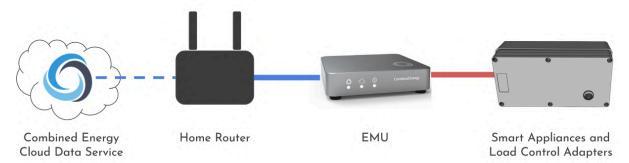
The EMU connects to the Internet to download weather and tariff data via either the home network or a dedicated cellular connection. Direct connection to the local network is made by connecting an Ethernet cable to the home router, or by joining to the home Wi-Fi via an optional Wi-Fi USB dongle. The USB expansion port also supports a range of commodity USB cellular modems for standalone operation.
