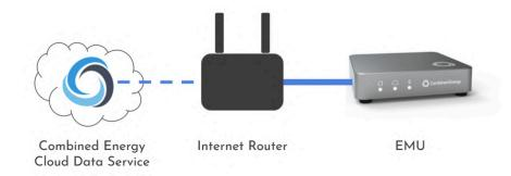
Use an Ethernet cable to connect the EMU to the Internet router.
