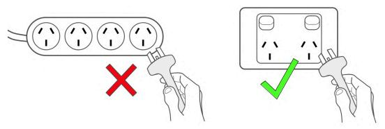
The socket-outlet shall be installed near the equipment and shall be easily accessible.
