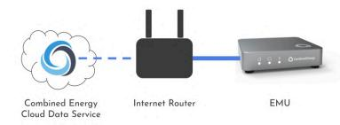
OPTION 2: Ethernet connection to a third-party Wi-Fi extender (extender joined to home Wi-Fi network)
